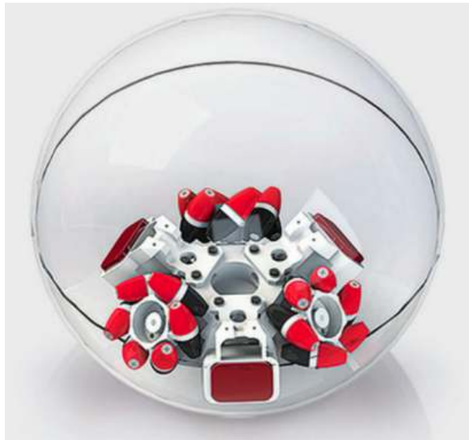
Figure 3.9: Concept of Swedish-wheel IDU by Karavaev et al. [35] [34]. The IDU holds three Swedish wheels and is therefore holonomic.
