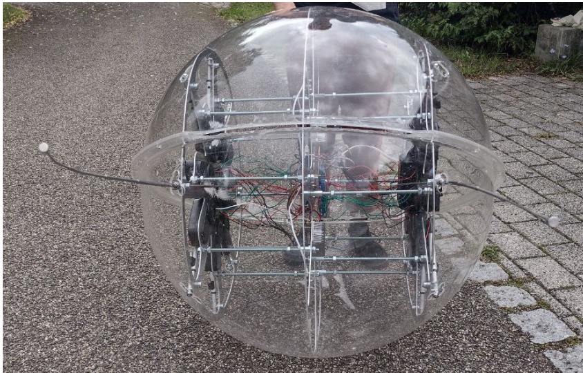
Figure 6.28: Deformed poles after pushing on gravelly ground. The deformation happened due to their own force.
