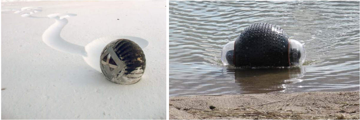
Figure 3.5: Rotundus (left) and the successor GroundBot (right), originally investigated by Ångström Space Technology Center, now by a Swedish company [36][24]. Both use an internal rotatable weight for locomotion. The design focuses on durability in rough terrains. The Groundbot has two acrylic domes on each side for camera sensors.
