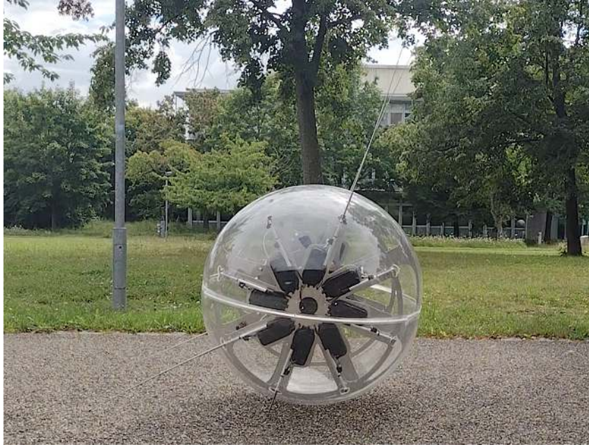
Figure 6.26: Endpose of the sphere outside with the push and leverage approach and stabilizing. The force of the poles is not enough for further rotation.
